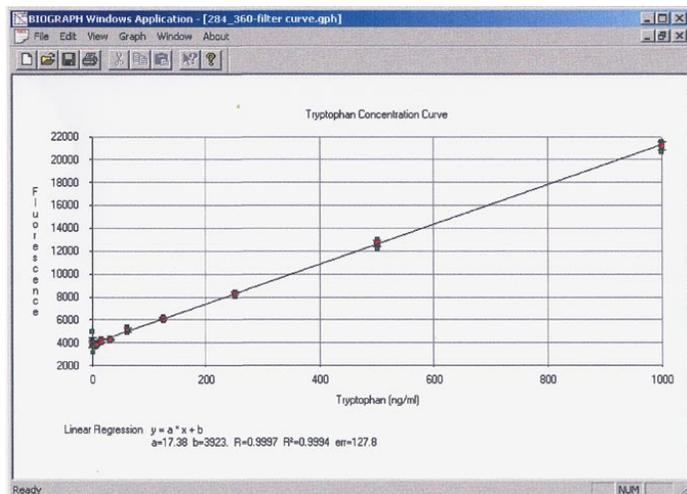
**Figure 8. Tryptophan Concentration Curve.** Dilution of tryptophan ranging from 0 to 1000 ng/ml were aliquoted into the microplate and the fluorescence measured. Using the UV excitation capabilities of the xenon-flash lamp, tryptophan in solution can be detected using an excitation wavelength of 284 nm and a 360/40 emission filter.
