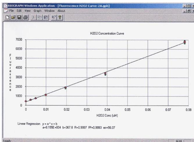
**Figure 5. Hydrogen Peroxide Fluorescence Calibration Curve.** Hydrogen Peroxide samples (in duplicate) ranging from 0 to 0.08  $\mu M$  were reacted with HRP and Amplex Red reagent and the fluorescence measured with a Synergy HT using a 530/25-excitation and a 590/35-emission filter. The subsequent data were plotted and linear regression analysis performed using KC4 Data Reduction Software.
