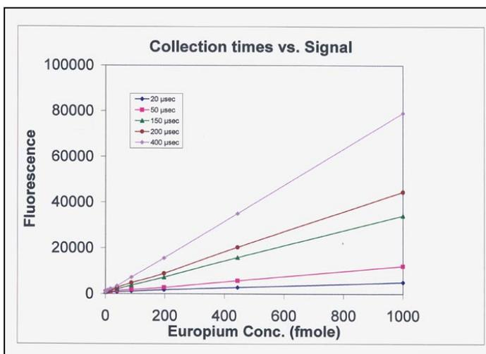
**Figure 7. Effect of Collection time on the fluorescence signal of Europium Chelate.** Using a Synergy HT, the fluorescence of the same microplate with a series of europium dilutions was measured repeatedly with a delay time of 20  $\mu$ sec and increasing collections times ranging from 20  $\mu$ sec to 400  $\mu$ sec. The reader was controlled and the data collected using KC4 data reduction software. After collection, the data were exported to Microsoft® Excel and plotted.
