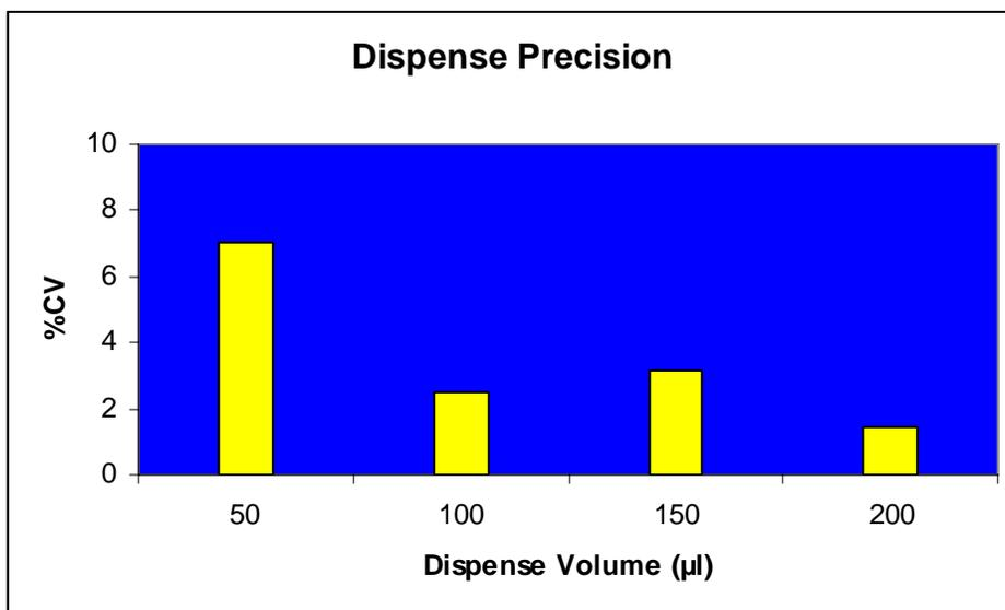
**Figure 4. Dispense Precision with Microscint 40 Scintillation Cocktail.** Various volumes of Microscint 40 cocktail were dispensed into 1 x 8 strips in a microplate frame using the  $\mu\text{Fill}$  Reagent Dispenser. Using gravimetric measurements, the mean dispense volumes of the wells for each 1 x 8 strip were calculated
