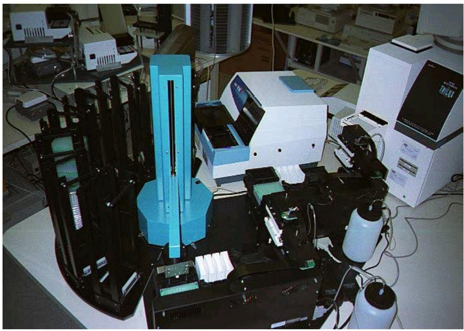
Figure A: Bench layout of PlateCrane XL, dual Precision 2000 pipetting systems, and three interchangeable detectors.
