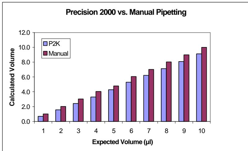
Figure 5. Comparison of dispense accuracy between the Precision 2000 and manual pipetting. The indicated volumes of yellow dye solution were pipetted into plate wells partially filled with 100µl of diluent. Absorbance values were then interpolated against a previously prepared standard curve. The manual data represents the mean of eight determinations, while the Precision 2000 data represents the mean of 96 wells.
