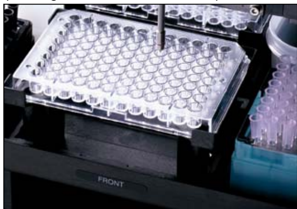
Figure 3. Single-Channel Dispenser filling an isolated well of a 96-well microplate.
