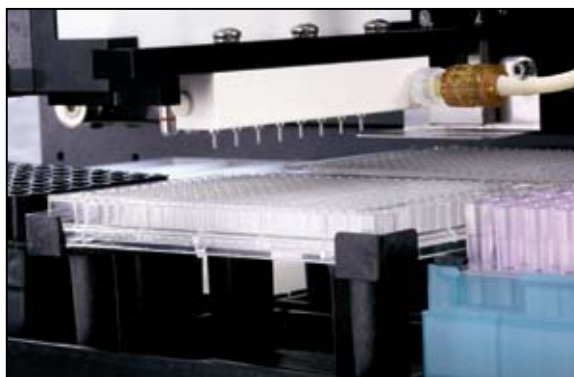
Figure 4. 8-Channel Bulk Dispenser filling a 384-well microplate. The Precision XS is available with an autoclavable and 100% DMSO compatible bulk reagent dispenser.
