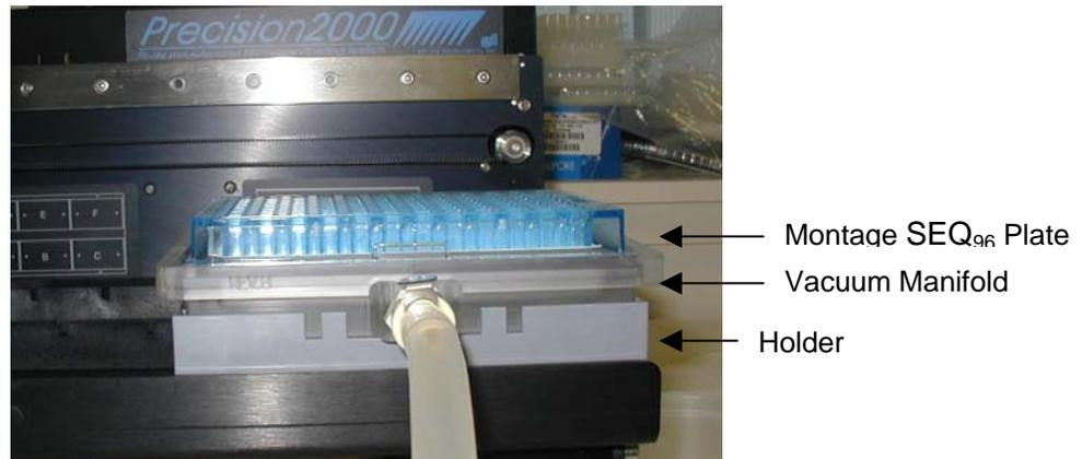
**Figure 4. Vacuum manifold and holder with a Montage SEQ<sub>96</sub> plate.** The vacuum manifold is situated on the deck using a multipurpose holder (P/N 7112110), which has been designed among other things to hold the vacuum manifold. The Montage SEQ<sub>96</sub> plate is situated on the vacuum manifold.
