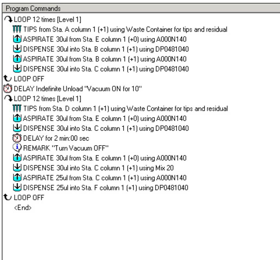
Figure 3. Programming Steps used by the Precision™ Microplate Pipetting System.
