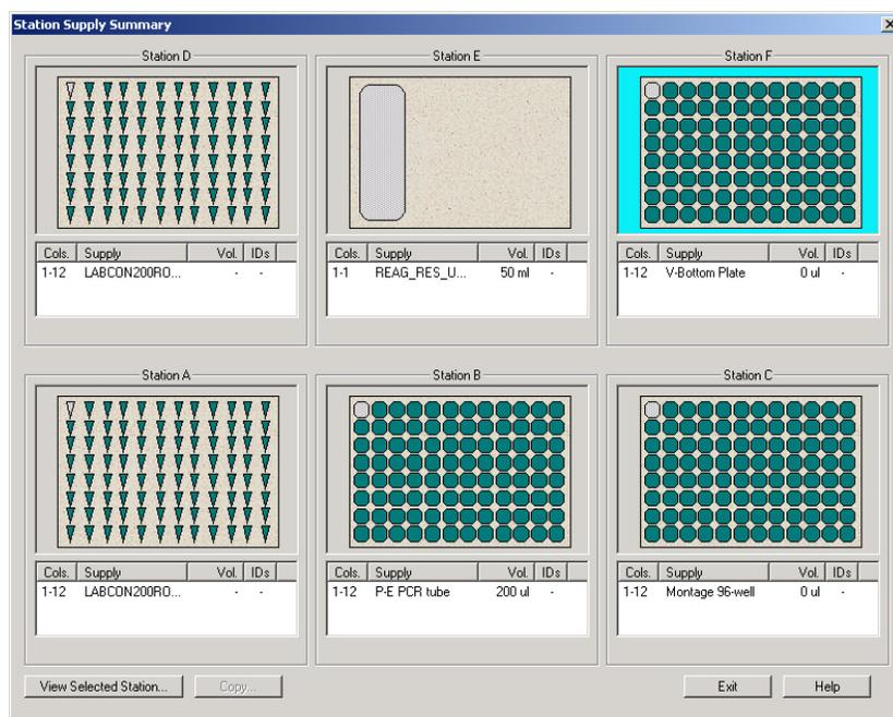
**Figure 2. Deck Layout of the Precision™ Microplate Pipetting System.** The positions of the necessary hardware on the deck, as described in Figure 1, are defined in the Precision Power™ Software (BioTek Instruments). A graphical representation is then provided within the software.
