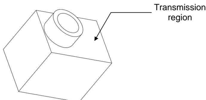
**Figure 2. Bio-Cell™ with approximate orientation for filling.** Note that the port opening is tilted upward so that the Bio-Cell can be completely filled.
