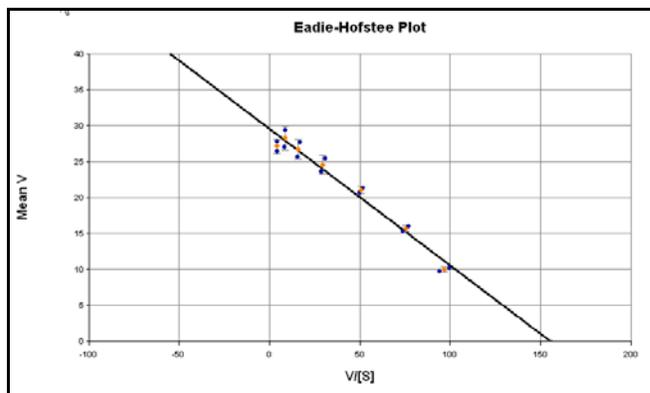
**Figure 6. Eadie-Hofstee Transformation of the substrate concentration vs. reaction velocity.** Reaction velocity ( $v$ ) was plotted against velocity divided by substrate concentration ( $v/[S]$ ) and linear regression analysis performed. Note that the y-intercept "b" defines the  $V_{max}$  of the reaction, while the slope "a" defines  $-K_m$ .
