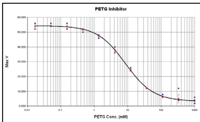
**Figure 8. Effect of PETG inhibitor concentration on  $\beta$ -galactosidase  $V_{max}$ .** Increasing concentrations of PETG were added to samples containing 0.25 U/ml  $\beta$ -galactosidase enzyme and the samples, kinetic readings at 420 nm every 30 seconds taken.  $V_{max}$  values were calculated for each inhibitor concentration and plotted using a 4-parameter logistic fit. Note that the ordinate axis (PETG concentration) is expressed in a log scale.
