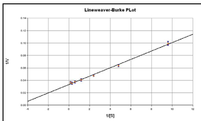
**Figure 7. Lineweaver-Burk or double reciprocal plot of velocity versus substrate concentration.** Reciprocals of experimentally determined reaction velocity ( $1/v$ ) were plotted against the reciprocal of substrate concentration ( $1/[S]$ ) and linear regression analysis performed. The y-intercept "b" defines the reciprocal of  $V_{max}$ , while the slope "a" is equal to  $K_m$  divided by  $V_{max}$ .
