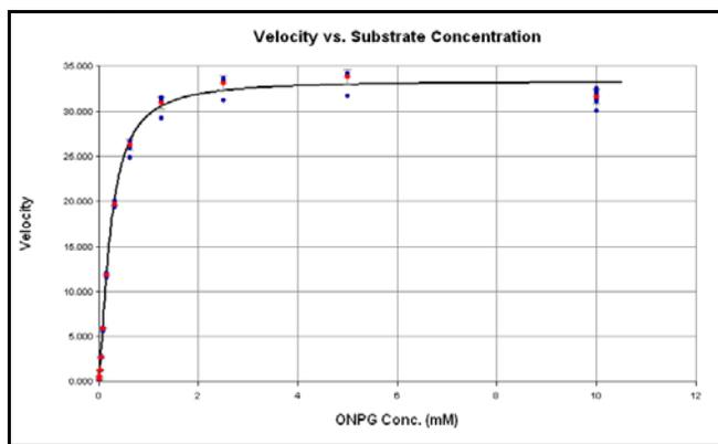
**Figure 5. Effect of substrate concentration on enzyme velocity.** Increasing concentrations of ONPG were reacted with 0.25 U/ml  $\beta$ -galactosidase enzyme and the absorbance determined kinetically. The average velocity was then plotted against the ONPG substrate concentration using a 4-Parameter logistic fit to describe the data. The Michaelis-Menten equation values for  $K_m$  and  $V_{max}$  were then calculated using Gen5.
