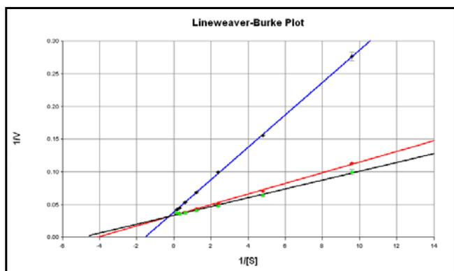
**Figure 10. Lineweaver-Burk plot of  $\beta$ -galactosidase activity in the presence of PETG inhibitor.** Double reciprocal plot of the data presented in Figure 9. The black line represents samples with 0 mM PETG, while the red line plots 0.167 mM PETG and the blue line plots 1.67 mM PETG. Linear regression of the three data sets were plotted and overlaid using Gen5.
