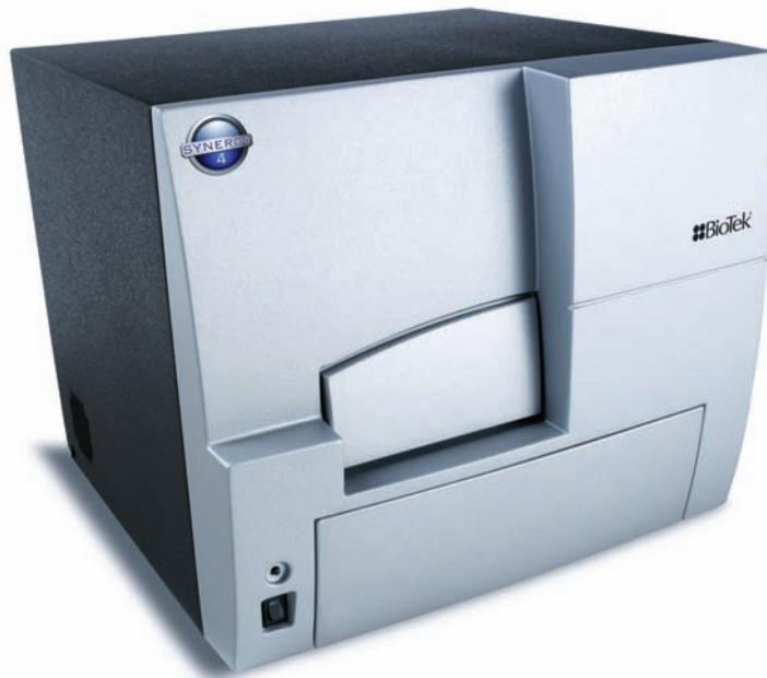
Figure 1 Synergy 4 multidetection microplate reader.
