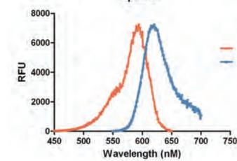
Figure 13 – Spectral Scanning Experiment. An excitation and emission spectral scan of the Alexa594 Tracer from the Transcreener ADP<sup>2</sup> FI Assay was performed using the monochromator system on the Synergy H1. Excitation scans were performed from 450-650nm in 1nm increments, with emission set at 680nm. Emission scans were performed from 550-700nm in 1nm increments, with excitation set at 520nm.
