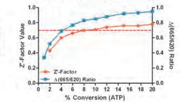
Figure 12 – TR-FRET Assay: Effect of ATP Conversion on Assay Quality. A. Assay window and Z'-Factor scores improve using the TR-FRET assay with increasing ATP conversion. B. Excellent Z'-Factor scores are able to be achieved with as little as 8% conversion of ATP to ADP.
