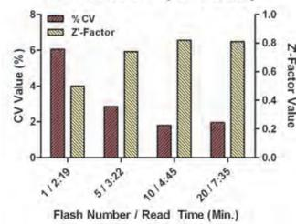
Figure 5 – FP Assay: Flash Number Effect on Data Variability and Quality. Additional flashes decrease the variability within measurements. Therefore, due to the Z'-Factor equation, this phenomenon increases the final Z'-Factor score for that data set.
