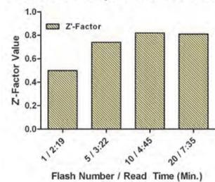
Figure 4 – FP Assay: Flash Number Effect on Z'-Factor Data Quality. Excellent Z' values can be achieved using as little as 5 flashes. Therefore high data quality can be seen while maintaining high-throughput.
