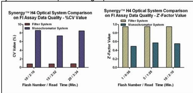
**Figure 10.** FI Assay Data Quality vs. Flash Number (Filter and Monochromator System Comparison)
