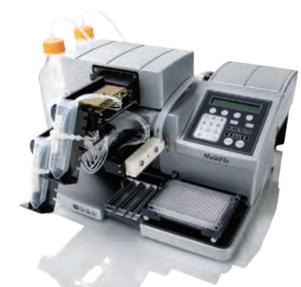
MultiFlo™ Microplate Dispenser peri pump cassettes were used for seeding cells in media to assay plates, and all assay reagent dispenses using a low flow rate and the BioTek Liquid Handling Control™ (LHC™) software. The MultiFlo and ELx50 Washer fit comfortably side-by-side in a 36-inch laminar flow hood. The cassettes are fully autoclavable adding to the compatibility of the MultiFlo for cell based work.
