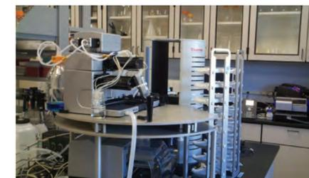
**Figure 8** – Images of Modular Robotic Assay System. Photo depicts complete modular automated system with random access stacks, Mezzanine Table, 405 Touch Microplate Washer and MultiFlo Microplate Dispenser. The Eon Microplate Spectrophotometer (not seen) is located on other side of Orbitor RS plate mover
