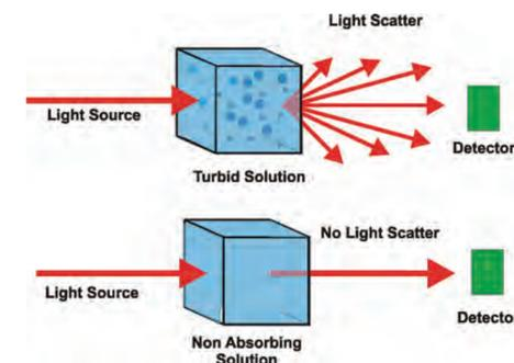
Figure 1 – Basis of 600 nm turbidimetry measurements.
