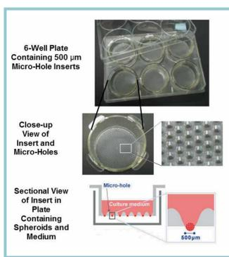
Figure 1. MPC 500 6 Micro-hole hanging drop insert design for spheroid formation.
