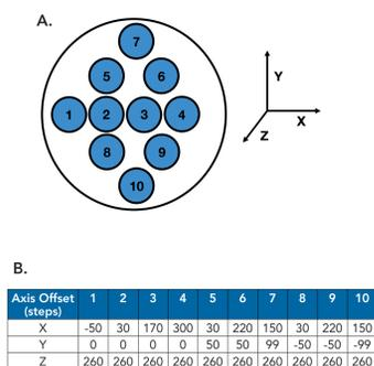
Figure 2. Automated hMSC Dispensing. (A) Multi-Flo FX RAD module hMSC dispense pattern; and (B) liquid handling control step offsets for RAD module dispensing of hMSC suspension.
