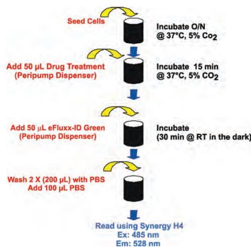
**Figure 2** – Schematic of the automated eFlux-ID Green assay process carried out by the EL406 Washer Dispenser (Red text) and Synergy™ H4 Reader (Blue text).
