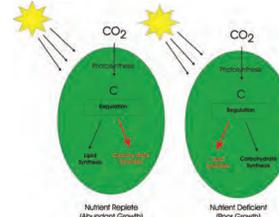
Figure 7 – Nutrient induced shift of Algal cell Energy Storage. Nutrient deficiency results in a change from carbohydrate and polar lipid production to non-polar triglyceride lipids.
