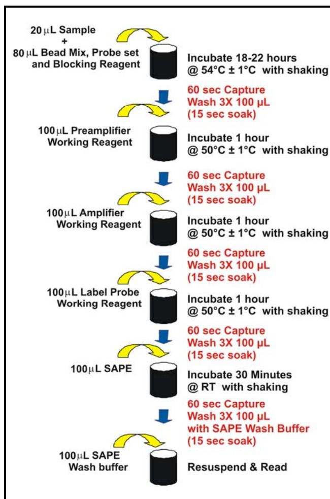
**Figure 3. QuantiGene Plex 2.0 Assay Protocol using an ELx405 Select Magnetic Bead Washer.** Using an initial soak time of 60 seconds to capture the beads, wash programs consisting of a series of aspiration and dispense steps each followed with a soak under magnetization were performed.
