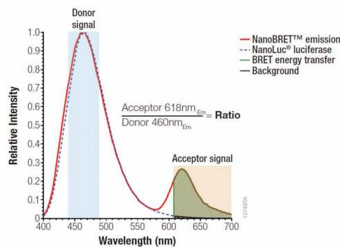
**Figure 2 – NanoBRET<sup>®</sup> Spectra.** Spectra of NanoLuc<sup>®</sup> emission at 460 nm and fluorescent emission at 618 nm of HaloTag<sup>®</sup> NanoBRET<sup>®</sup> ligand. NanoBRET<sup>®</sup> ratio calculation based on donor/acceptor emission.
