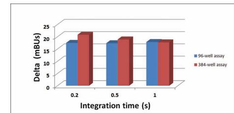
**Figure 5. Synergy Neo2 reader settings optimization.** The delta between mBU response from treated and untreated cells at various integration times and gain settings were compared to determine optimal reader settings.
