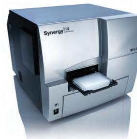
The Synergy H4 combines a filter-based and monochromator-based detection system. The filter-based system and Xenon flash lamp was used to detect the 530 nm fluorescent emission using Ex: 485/20 and Em: 528/20 filters, along with a 510 nm cut-off mirror.
