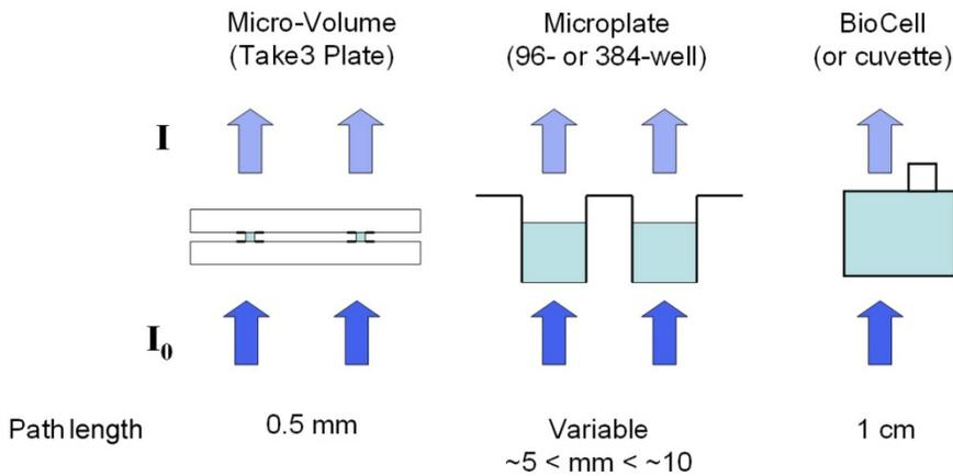
**Figure 1.** Multi-Volume analysis capabilities in a microplate reader.
