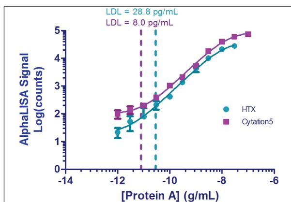
**Figure 2. Protein A Standard Curve.** A 12-point dilution series of the positive control was prepared ranging from 100,000 - 0.3 pg/mL. Twelve background points were used to calculate LDL.
