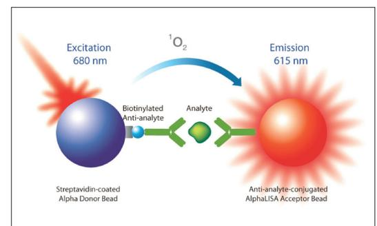
**Figure 1.** Assay schematic for AlphaLISA homogeneous proximity assay principle for the detection of analyte in biotherapeutic products. Upon excitation, the AlphaLISA donor bead generates singlet oxygen molecules. If the acceptor bead is in close proximity due to the creation of a sandwich immunoassay, the singlet oxygen molecules will trigger a cascade of energy transfer in the acceptor bead, resulting in a sharp peak of light emission at 615 nm.
