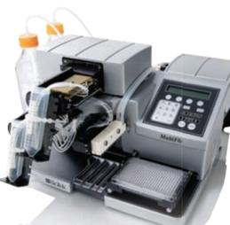
MultiFlo™ Microplate Dispenser peristaltic pump driven 5 $\mu$ L and 10 $\mu$ L cassettes were used for seeding cells in media to tissue culture plates, and all assay reagent dispenses. An 8 point cell serial dilution was dispensed simultaneously to a tissue culture plate using a single cassette (shown Figure 2). The peri pump cassettes are fully autoclavable adding to the versatility of the MultiFlo design.
