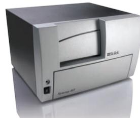
Synergy™ HT Multi-Mode Microplate Reader was used to detect Raw Fluorescence Units using a filter set of 540/25 for excitation and 590/20 for emission. Following an Auto Sensitivity test on a high well for the assay, the setting of 46 was used for all experiment detection sensitivity.
