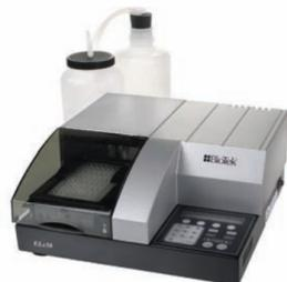
ELx50™ Microplate Strip Washer was used for both cell and assay wash steps. Settings were optimized for minimal cell loss during aspiration and buffer dispense. The instrument fits comfortably under a 36-inch laminar flow hood next to the MultiFlo™ Microplate Dispenser (shown Figure 2).
