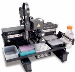
Precision™ XS Microplate Sample Processor was used for all assay serial dilutions and transfers to the assay plate for the intra- and inter-variability runs.
