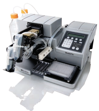
Figure 4 – MultiFlo ™ Microplate Dispenser. The dispenser offers fast, accurate non-contact plate dispensing capabilities through its two peristaltic and two syringe pumps, with volumes ranging from 1-3000 µL. The peristaltic pump on the instrument was used to dispense cryopreserved cells, and detection solution to the LV384-well assay plates.
