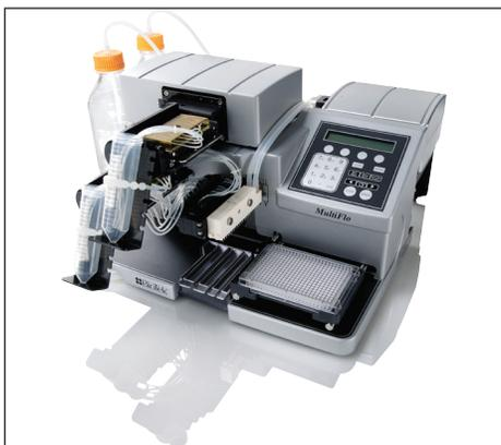
Figure 3. MultiFlo™ Microplate Dispenser.
