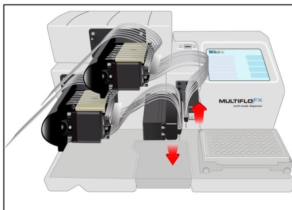
Figure 1. MultiFlo FX Multi-Mode Dispenser equipped with the AMX Automated Media Exchange module, showing aspirate (right arrow) and dispense (left arrow) heads.
