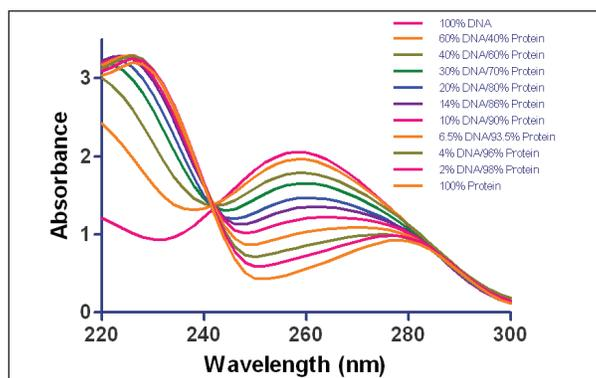
**Figure 3.** Absorbance spectral scans of purified dsDNA, protein or a mixture. Samples contained purified herring sperm dsDNA, BSA protein or a DNA/protein mixture at varying ratios (w/w). Measurements were taken at 1 nm intervals at wavelengths ranging from 220 to 300 nm. Data normalized to a 1 cm path length.
