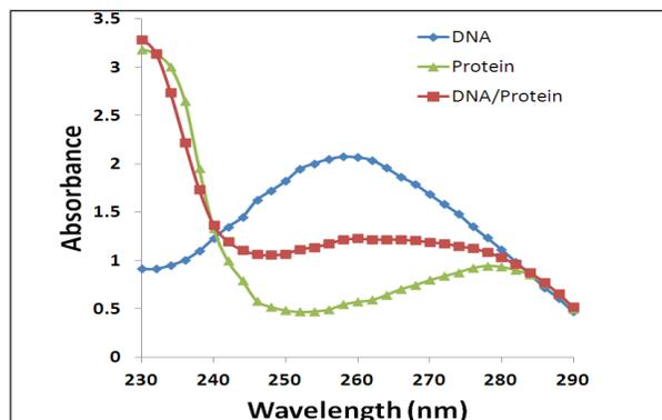
**Figure 2.** Biomolecule spectral data comparison. Typical absorbance profiles of purified dsDNA, BSA protein, and a complex mixture containing 1:10 DNA/protein (w/w). Spectral analysis of samples was performed at 1 nm increments from 230 nm to 290 nm. Data normalized to a 1 cm path length.
