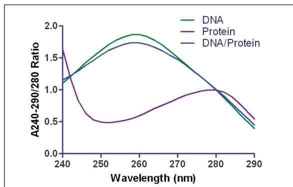
**Figure 4.** Typical  $A_{280}$  ratios associated with samples of biomolecules. Samples contained purified dsDNA, protein or a DNA/protein mixture (60%/40%) (w/w). Measurements were taken at 1 nm intervals at wavelengths from 240 to 290 nm. The  $A_{280}$  ratio was then calculated by dividing each wavelength measurement by the  $A_{280}$  measurement for each sample. Data has been normalized to 1 cm.
