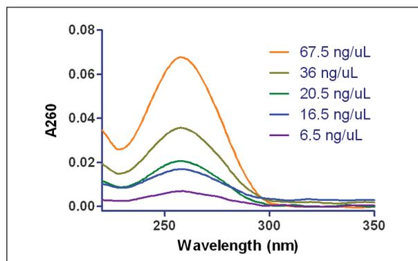
**Figure 1.** Micro-volume spectral scanning analysis. Spectral scanning micro-volume analysis representing duplicate 2 µL samples of dsDNA in TE buffer using the Synergy H4 and Take3 Micro-Volume Plate. The data indicates the ability to perform micro-volume spectral analysis on sample in the low ng/µL range. (Values represent blanked data normalized to a 0.5 mm path length).
