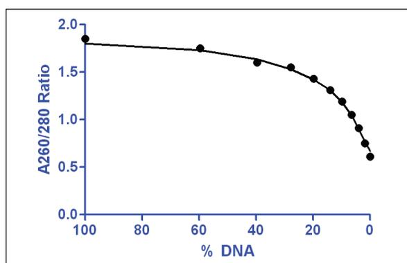
**Figure 5.**  $A_{260}/A_{280}$  ratios associated with increasing protein contamination of DNA. Samples contained purified herring sperm dsDNA with increasing concentrations of BSA ranging from 40-100% (w/w). Measurements were taken at 260 to 280 nm. The  $A_{260}/A_{280}$  ratio was then calculated for each DNA/protein mixture. Data has been normalized to 1 cm.
