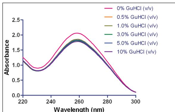
**Figure 6.** Spectral analysis of DNA: GuHCl contamination. Spectral analysis of herring sperm dsDNA spiked with increasing concentrations of guanidine hydrochloride. Data has been normalized to a 1 cm pathlength.
