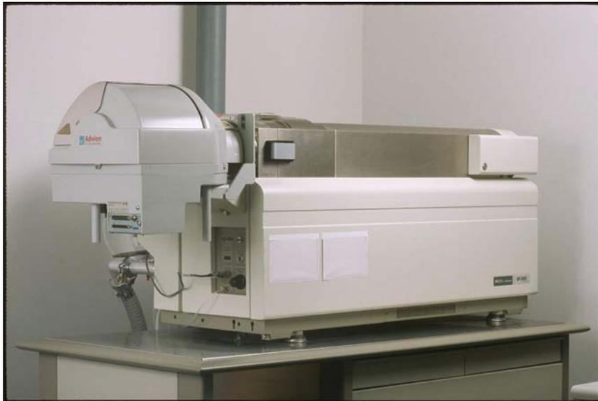
**Figure 3. NanoMate 100 Automates Nanoelectrospray System attached to a Mass Spectrometer.**
