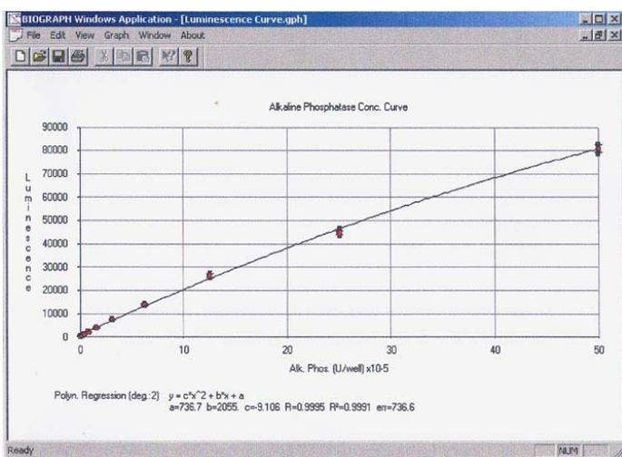
**Figure 9. Alkaline Phosphatase Concentration Curve.** Dilutions of alkaline phosphatase ranging from 0 to 50 x 10<sup>-5</sup> DEA units per well were aliquoted into microplates and CSPD/Sapphire II chemiluminescence reagent added. The luminescence of each sample was determined after a 30-minute incubation.
