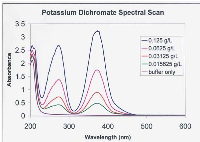
**Figure 4. Spectral Scans of Potassium Dichromate Solutions.** Spectral scans from 200 nm to 600 nm in 1 nm increments were performed on several dilutions of potassium dichromate dissolved in an aqueous solution of 0.05N KOH. Data from each spectral scan were exported to Microsoft® Excel and plotted.
