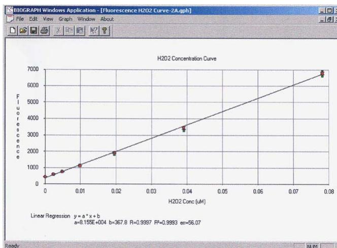
**Figure 5. Hydrogen Peroxide Fluorescence Calibration Curve.** Hydrogen Peroxide samples (in duplicate) ranging from 0 to 0.08 μM were reacted with HRP and Amplex Red reagent and the fluorescence measured with a Synergy HT using a 530/25-excitation and a 590/35-emission filter. The subsequent data were plotted and linear regression analysis performed using KC4 Data Reduction Software.
