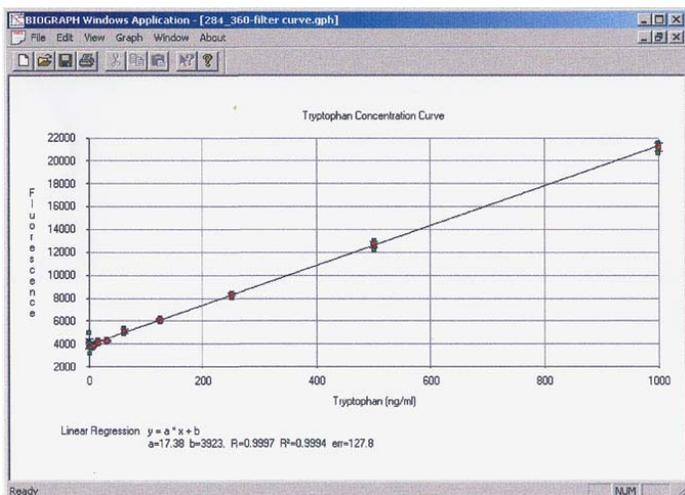
**Figure 8. Tryptophan Concentration Curve.** Dilutions of tryptophan ranging from 0 to 1000 ng/ml were aliquoted into the microplate and the fluorescence measured. Using the UV excitation capabilities of the xenon-flash lamp, tryptophan in solution can be detected using an excitation wavelength of 284 nm and a 360/40 emission filter.
