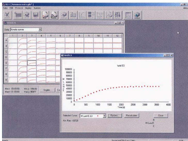
**Figure 10. Change in luminescence over time.** Luminescence determinations of alkaline phosphatase reactions ranging from 0 to  $1 \times 10^{-3}$  DEA units/well) were made kinetically every 2 minutes for 60 minutes. Note that one kinetic well has been enlarged. Reactions were prepared as described in materials and methods.
